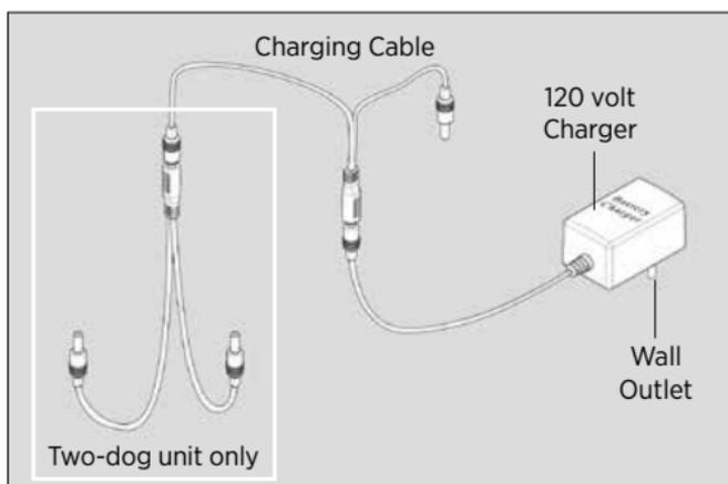
The Dogtra 2300NCP uses a lithium polymer battery. Recharge the unit if the indicator light is red or does not come on, the transmitter LCD shows only 1 bar on the indicator, or the system will not stay on when any button is pressed.
