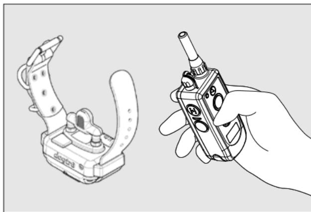
1. Turn on the receiver by placing the magnetic red dot on the back of the transmitter to the red dot on the receiver. The indicator light will come on for a moment then blink once every 4 seconds, showing that the receiver is ready to use (the receiver needs to be charged if the indicator light is red).
