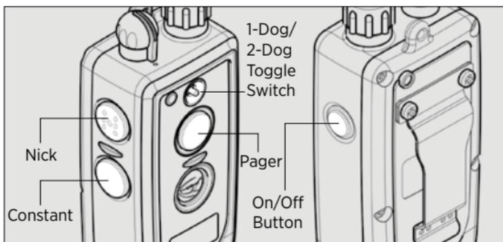
The transmitter for the 2300NCP EXPANDABLE unit has four buttons and a toggle switch on the transmitter (one on the face of the transmitter, two on the left side, and one on the right side).
